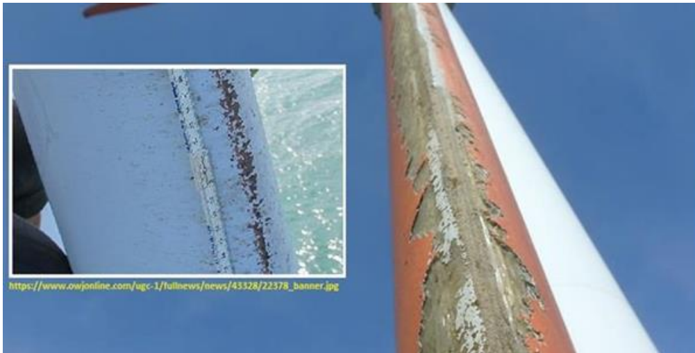
Figur 8: Leading Edge Erosion (LEE). Pedestal
